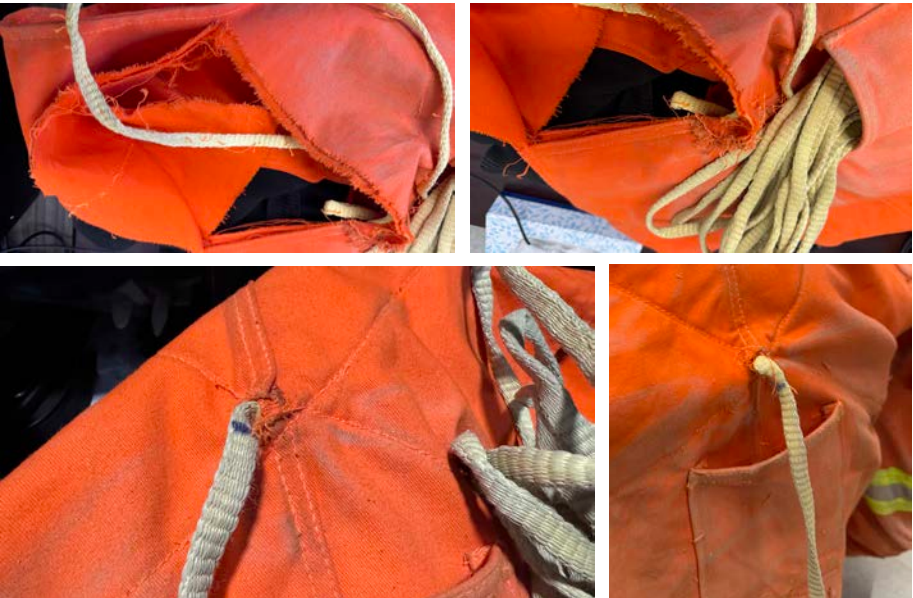
Damage Shown After Repeated Rescue Load Testing
