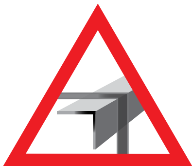
Global Sharp Edge symbol – Radius as sharp as .005 in. (.13mm)
